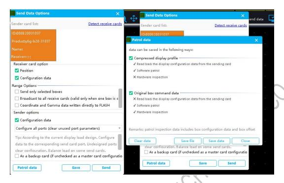
Send the display screen connection file in the complex screen adjustment interface of the upper computer screen configuration interface, and then click on the adjacent inspection data to save the data. For internal storage inspection, you can choose the inspection type: receiving card, sending card, all; You can choose the number of inspections, only the receiving card can conduct unlimited inspections, and sending cards can only be selected once; Cure after inspection.
